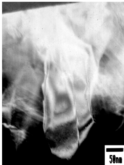
Figure 3. A \text{NH}_3 -MBE specimen: a GaN layer showing a rough top surface (thickness: 500 nm).
